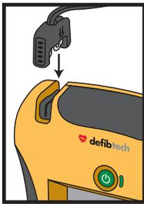
Insert the connector end of the defibrillation pad cable into the pads connector socket on the top-left corner of the DDU-2000 Series AED as shown at left. Insert pads connector firmly until it is fully seated in the unit. The connector will only fit in one way – if the connector does not fit, rotate the connector before trying again.
