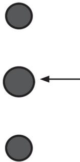
To check the status of the AED when the unit is off, press the **center softkey button**. The display screen will show unit status, battery pack status, and pad status. After a short period of time, the display screen, and the unit will turn off.
