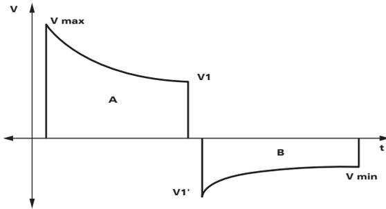
The waveform is adjusted to compensate for measured patient impedance. Nominal phase times and energy delivered are shown in the tables below.
