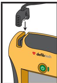
Connect pads to unit, if not already connected. Follow AED voice and display instructions. The DDU-2000 Series AED is designed to be stored with the defibrillation pads connector attached to the unit, while the pads themselves remain sealed in their package. This reduces the time needed to set up and start treatment in an emergency.
