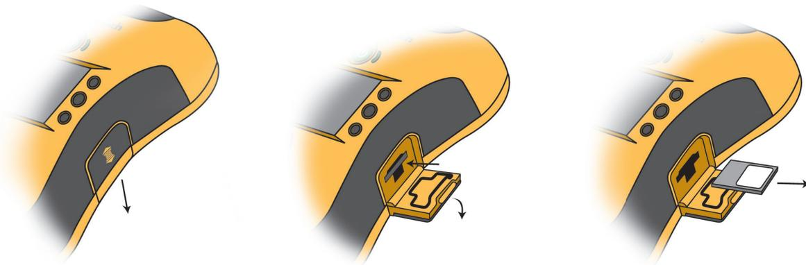
To remove the DDC card, ensure the AED is OFF. Locate the data card/USB port access door on the right-hand side of the unit. Open the data card/USB port access door by slightly pushing and then sliding the door down to release the latch. The door will spring open. To remove the DDC card, press the card in as far as it will go, and then release. Upon release, the DDC card will be partially ejected and can be removed by pulling the DDC card the rest of the way out.
