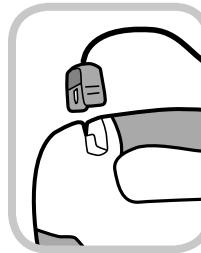
Insert the connector end of the defibrillation pad cable into the pads connector socket on the top-left corner of the DDU-100 AED as shown at left. Insert the pads connector firmly until it is fully seated in the unit. The connector will only fit in one way – if the connector does not fit, rotate the connector before trying again.
