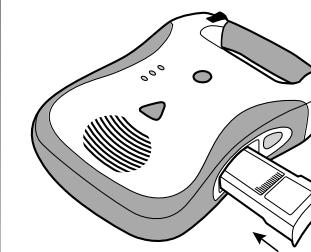
When the battery pack is installed, the AED will turn on and run a battery pack self-test. Wait for the test to complete and for the unit to turn off.
