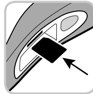
**Note:** A DDC card is not required for the AED to operate. Even if a DDC card is not installed, relevant event information will still be recorded internally. The AED will still operate properly even after a "replace data card" message.
