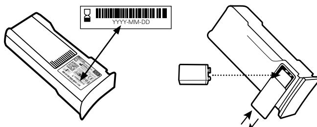
Check battery pack expiration date as shown. Record battery pack expiration date for future reference.
