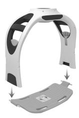
To remove the Frame, push in on the two backboard release levers and lift the Frame off of the Backboard. The latches may be released together or one at a time.
