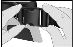
The Stabilization Strap's length can be adjusted by either pulling on the ends of the Main Strap (to tighten) or feeding the strap back through the buckle connector (to loosen), as shown in the illustrations below. Be sure that the Stabilization Strap is sufficiently tightened so that the RMU-2000 ACC's correct position over the patient's chest can be maintained.
