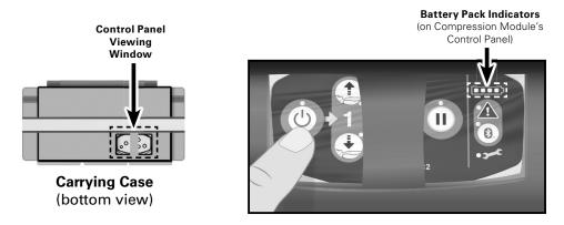
The Battery Pack installed in the Compression Module can be charged while remaining inside the Carrying Case. To do this, open the Charging Access Flap located on the back of the Carrying Case and connect the AC Adapter plug to the external power input jack on the Compression Module, as shown here:
