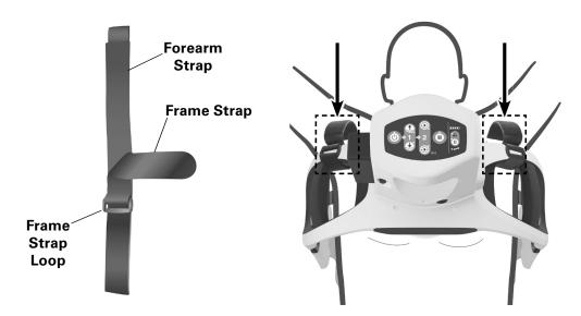
The Patient Wrist Straps are designed to attach a patient's arms to the RMU-2000 ACC for ease of transporting the patient and the RMU-2000 ACC. As shown in the above left illustration, each Patient Wrist Strap is comprised of two main strap sections: a Frame Strap that attaches to the Frame and a Forearm Strap that wraps around the patient's wrist.
