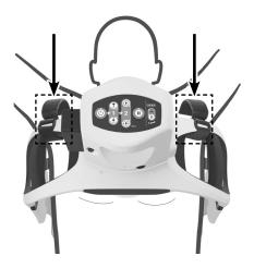
As shown in the illustration above, when attaching the Frame to the Backboard, the Patient Wrist Straps can be oriented towards the patient's head to maintain access to the Frame's Backboard Release Levers or on the opposite side of the Frame as appropriate.
