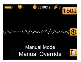
**Manual Mode** - Displays ECG and allows defibrillation energy selection (25-200J) with charge, shock, and disarm control.
