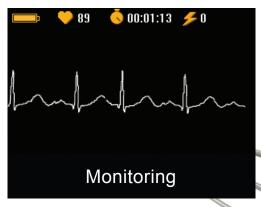
**ECG Mode** - Displays ECG waveform using an optional 3-wire (LEAD II) ECG adaptor cable.
