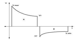
The waveform is adjusted to compensate for measured patient impedance. Nominal phase times and energy delivered are shown in the tables that follow.
