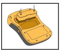
Before inserting the battery pack into the DDU-2000 Series AED as shown at left, ensure that the battery pack opening in the back of the AED is clean and clear of any foreign objects. Insert the battery pack into the opening in the back of the AED. Push the pack all the way in until the latch clicks. The battery pack will only fit in one
