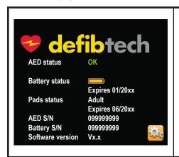
The AED Status Screen shown at left is used to provide a quick overview of the DDU-2000 Series AED's status and to display select information without turning the unit on in AED Mode.
