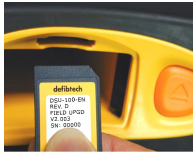
Figure 2: Insert the DSU-100 Software Upgrade Data Card as shown.
