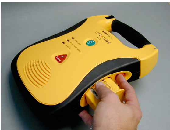
Figure 1 – Press the orange release button to eject the battery pack from the AED.
