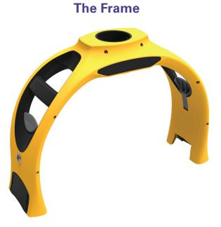
The single-piece Frame attaches to the Backboard and holds the Compression Module in position over the patient. With the Backboard attached, the Frame is designed to create a rigid structure that enables a consistent compression depth without unwanted flex or distortion during operation. The latches are self-centering and self-locking and are easy to match up with, and snap into, the Backboard.
