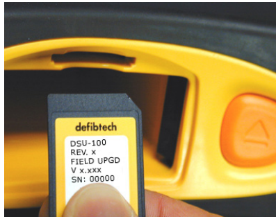
Figure 2: Insert the DSU-100 Software Upgrade Data Card as shown.
