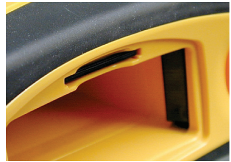
Figure 3: Push the card in until it clicks into place flush with surface as shown.
