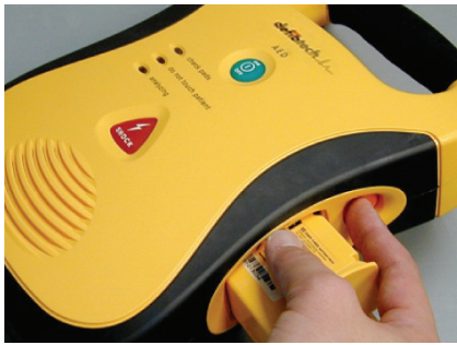
Figure 1: Press orange release button to eject the battery pack.
