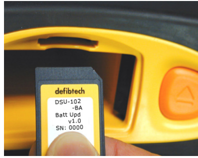
Figure 2: Insert the DSU-102 Battery Pack Update Data Card label side up as shown.
