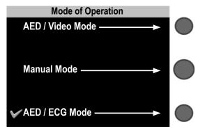
Mode of Operation screen (with corresponding softkey buttons)
