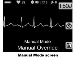
When charging is complete, press the flashing SHOCK button.
