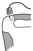
The *DDU-100* AED defibrillation/monitoring pads are supplied sealed in a pouch with the connector and part of the cable exposed. This allows the pads to be stored in a pre-connected state for rapid deployment during an emergency.
