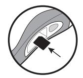
release. The DDC will be partially ejected and can be removed by pulling it the rest of the way out. To install a new DDC, insert the DDC, label side up, in the thin slot on the top of the opening for the battery pack. The card should click into place and be flush with the surface of the slot. If the card does not push in all the way, it may have been inserted upside down. In that case, remove the card, flip it over and try inserting it again.
