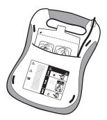
The pad package can then be stored in the pad storage slot in the back of the *DDU-100* AED. After connecting the pads connector to the unit, push the pad package, with the pictures on the package facing up and out, rounded end first, into the pad holder compartment on the back of the AED. When the pad pack is fully inserted, press the pad cable into the groove in the back of the unit to hold it in place and tuck any excess cable behind the pad package.
