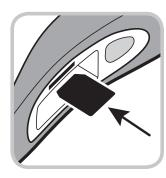
**Note:** A DDC card is not required for the AED to operate. Even if a DDC card is not installed, relevant event information will still be recorded internally. The AED will still operate properly even after a "replace data card" message.
