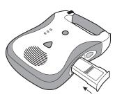
Ensure that the battery pack has not expired. Expired battery packs must not be used.
