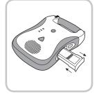
Within moments of insertion, the AED will turn on and run a battery pack insertion self-test. The unit will automatically shut off after the test is run. Afterwards, the Active Status Indicator on the top corner of the AED will periodically flash. If the indicator flashes green, the AED and battery pack are functioning properly, if the indicator flashes red, there is a problem. Refer to page 17 for more details on the meaning of the indicator.
