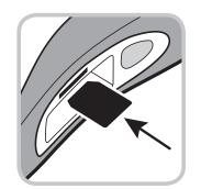
**Note:** A DDC card is not required for the AED to operate. Even if a DDC card is not installed, relevant event information will still be recorded internally. The AED will still operate properly even after a "replace data card" message.
