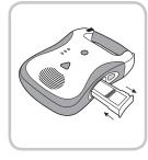
Within moments of insertion, the AED will turn on and run a battery pack insertion self-test. The unit will automatically shut off after the test is run. Afterwards, the Active Status Indicator on the top corner of the AED will periodically flash. If the indicator flashes green, the AED and battery pack are functioning properly, if the indicator flashes red, there is a problem. Refer to page 17 for more details on the meaning of the indicator.
