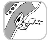
To remove the DDC card, press the card as far as it will go and then release. Upon release, the DDC card will be partially ejected and can be removed by pulling the DDC card the rest of the way out.
