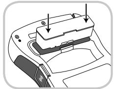
To remove the battery pack, push the battery pack eject release latch. After the battery pack is partially ejected, pull the battery pack out.
