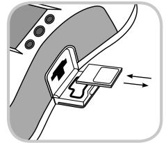
To remove the DDC card, press the card as far as it will go and then release. Upon release, the DDC card will be partially ejected and can be removed by pulling the DDC card the rest of the way out.
