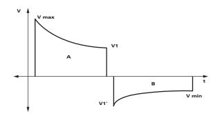
The waveform is adjusted to compensate for measured patient impedance. Nominal phase times and energy delivered are shown in the tables that follow.
