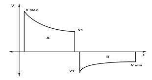
The waveform is adjusted to compensate for measured patient impedance. Nominal phase times and energy delivered are shown in the tables below.
