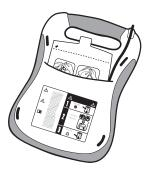
The pad package can then be stored in the pad storage slot in the back of the *DDU-120* AED. After connecting the pads connector to the unit, push the pad package, with the pictures on the package facing up and out, rounded end first, into the pad holder compartment on the back of the AED. When the pad pack is fully inserted, press the pad cable into the groove in the back of the unit to hold it in place and tuck any excess cable behind the pad package.
