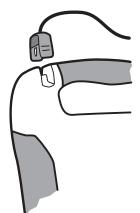
The *DDU-120* AED defibrillation/monitoring pads are supplied sealed in a pouch with the connector and part of the cable exposed. This allows the pads to be stored in a pre-connected state for rapid deployment during an emergency.
