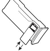
pack. The orientation of the battery contacts is shown in a picture on the inside bottom of the 9V battery compartment. Replace the 9V battery compartment door by reversing the process used to remove the door.
