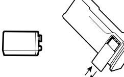
Ensure that the lithium 9V battery has not expired.
